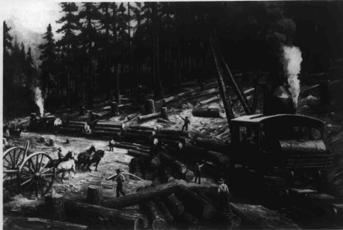
This oldtime logging show appeared on the October 1974 cover of the Journal of Forest History , painted by nationally known artist, Robert Lavin. A McGiffert loader hoists logs onto flatcars towed by a Shay locomotive at the far left, while a horsedrawn high wheels yards more logs to the landing.
